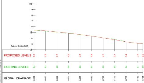
GEO\_HV-01\_ML\_0000\_M3\_CR-0002-A01 LONGITUDINAL SECTION 21 SCALE: H 1:500,V 1:100.
